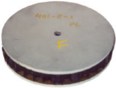
Figure 2.1: Stabilized Flatwise Compression Specimens (4" Diam.)
